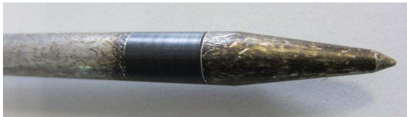
Soiled probe -> wrong measuring!
